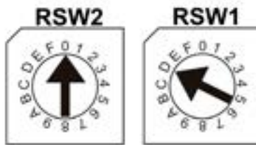
Figure 2) Example: If the address switches are set in this manner, RSW2 at 0 and RSW1 at D, the corresponding address in decimal number would be 13 (see table below).
