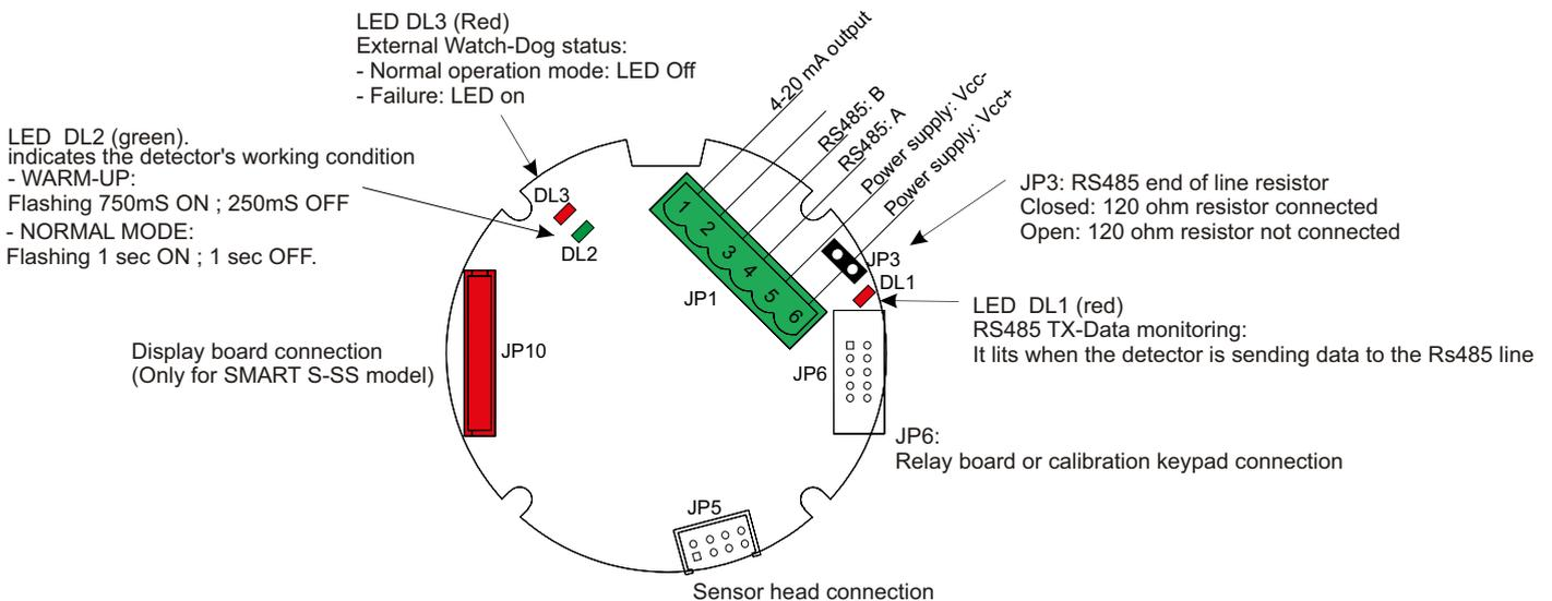
Figure 1) Detector circuit layout without HART module
