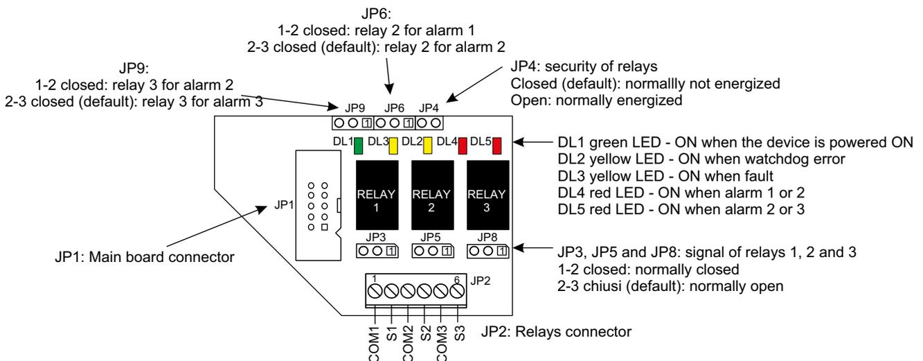
Figure 4) 3 relays board
