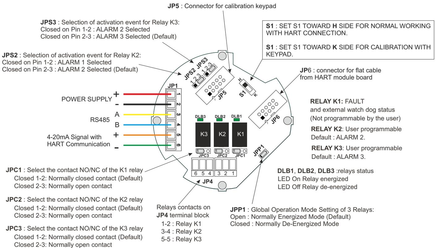
Figure 2) Detector circuit layout with HART module
