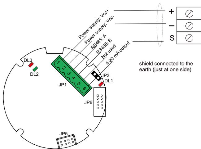
Figure 3) Connection scheme for the 4-20 mA output
