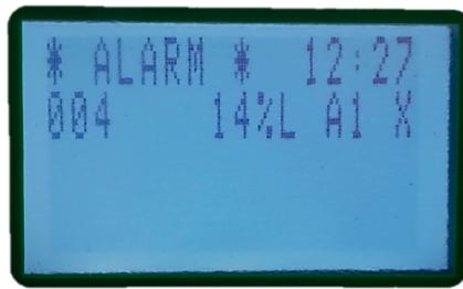
Figure 22) Screen in Alarm status
