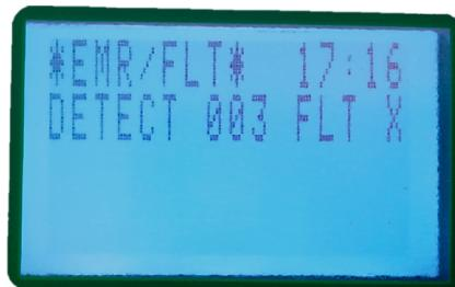
Figure 24) Screen in Fault status
