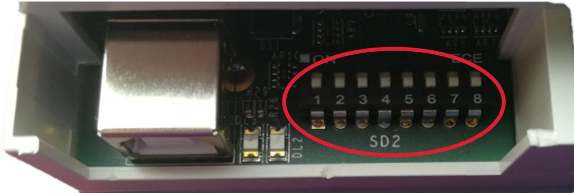
Figure 7) Dip switch series for baud rate settings
