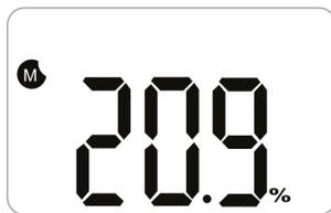
Following activation the device will operate in Gas Measurement Mode. The remaining sensor life (default setting) or gas concentration (configurable option) will be displayed on the screen. Oxygen concentration is displayed in percent by volume (%Vol) and toxic concentration is displayed in parts per million (PPM).
