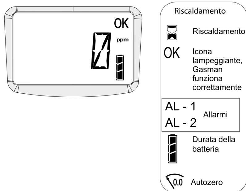
The sensor channel will display the current value of the gas being monitored and the unit of measurement, the 'OK' symbol will flash indicating unit is working correctly. Familiarise yourself with the gas being monitored in your unit. Ensure you understand site health and safety procedures. For information on Peak and TWA readings, go to section 2.4.
