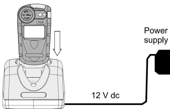
The Gasman should normally be switched off for charging. During charging the red LED on the front of the charger unit will be lit. When charging is complete the red LED is extinguished.
