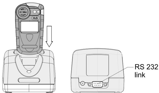
Gasman can be connected to a PC using the single way charger unit with optional PC interface. The charger unit is fitted with a D-type 9 pin RS232 socket which is located at the rear of the charger, see diagram below. The PC requires Crowcon Portables PC software. A USB-RS232 adaptor is also available from Crowcon.
