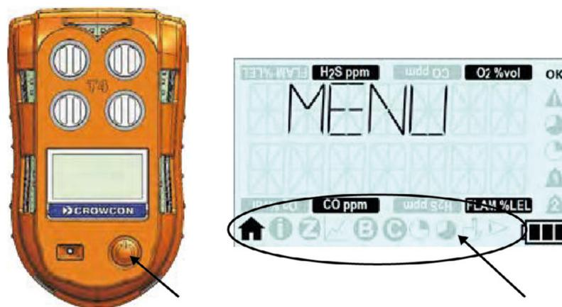
II Single click the operator button repeatedly to scroll right until the required menu icon is displayed and then double click the operator button to select the function.
