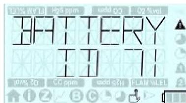
T4 will indicate a low battery alarm when the battery has a maximum of 30 minutes remaining life. This warning should be acknowledged immediately by pressing the operator button
