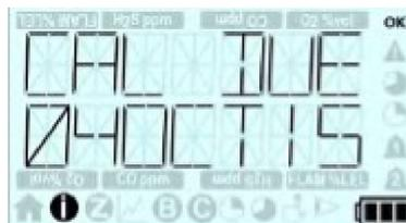
This screen then displays the date the T4's next calibration is due.
