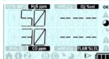
If a toxic sensor is fitted this screen displays the TWA configured alarm levels (see [Section 2.3.4](#)).
