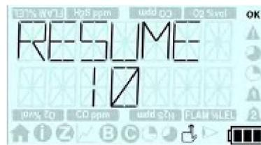
Upon start up, following the test screen, if T4 is switched on within 8 hours of being switched off, the screen shown right will be displayed for 10 seconds allowing the user to 'resume' if required. Simply click the operator button.
