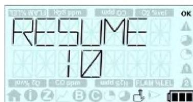
If T4 is switched on within 8 hours of being switched off, the following screen will be displayed for 10 seconds allowing T4 to retain TWA, STEL and peak readings (see Section 2.3.5 for more details on this feature). Simply press the operator button to retain, or do not click the operator button and allow countdown to expire.
