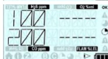
If a toxic sensor is fitted this screen displays the STEL configured alarm levels (see [Section 2.3.3](#)).
