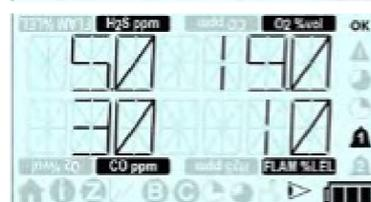
This screen displays the sensors configured lower alarm levels.
