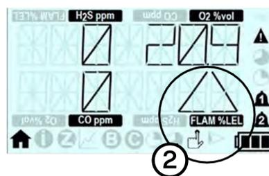
After the defined period the sensor can be re-activated by a single click of the operator button ② once the instrument is in a clean air environment.
