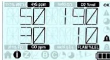
This screen then displays the sensors' configured upper alarm levels.
