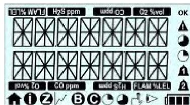
Firstly a test screen will be displayed showing all the possible LCD segments and icons turned on.
