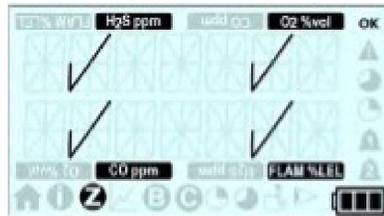
A successful zero of a channel will display a tick on the screen as can be seen, T4 will then automatically return to the home screen.
