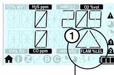
When the flammable gas exceeds the pellistor saver threshold, the detector will turn off the sensor for a minimum period of 200 seconds.
