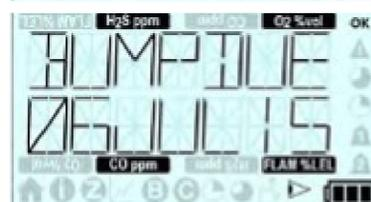
This screen displays the date the T4's next bump test is due. This screen will only be displayed if bump test is configured via Portables Pro 2.0.
