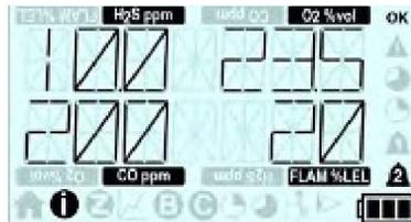
If a toxic sensor is fitted this screen then displays the STEL configured alarm levels (see Section 2.3.3).
