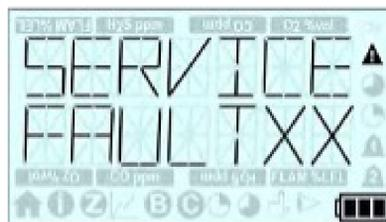
If T4 detects an internal fault that requires T4 to be returned for servicing 'Service' message as shown will be displayed on the screen, where 'XX' represents a specific fault ID code.
