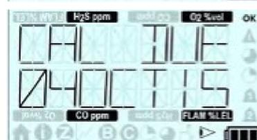
This screen displays the date the T4's next calibration is due
