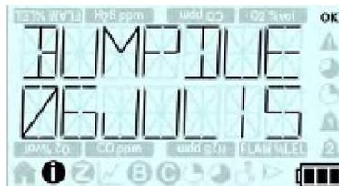
This screen then displays the date the T4's next bump test is due. This screen will only be displayed if bump test is configured via Portables Pro 2.0.
