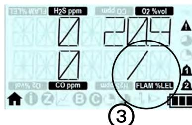
After a stabilisation time ③, if the gas level still exceeds the threshold then the sensor will be turned off and the cycle starts again.
