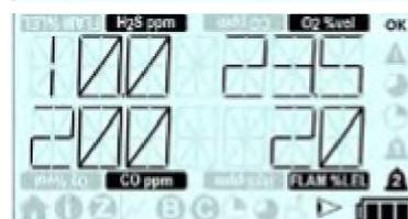
This screen displays the sensors configured upper alarm levels.
