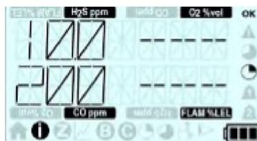
If a toxic sensor is fitted this screen then displays the TWA configured alarm levels (see Section 2.3.4)
