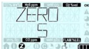
If configured to do so, the last screen is the autozero screen. This will operate as configured via Portables Pro 2.0.
