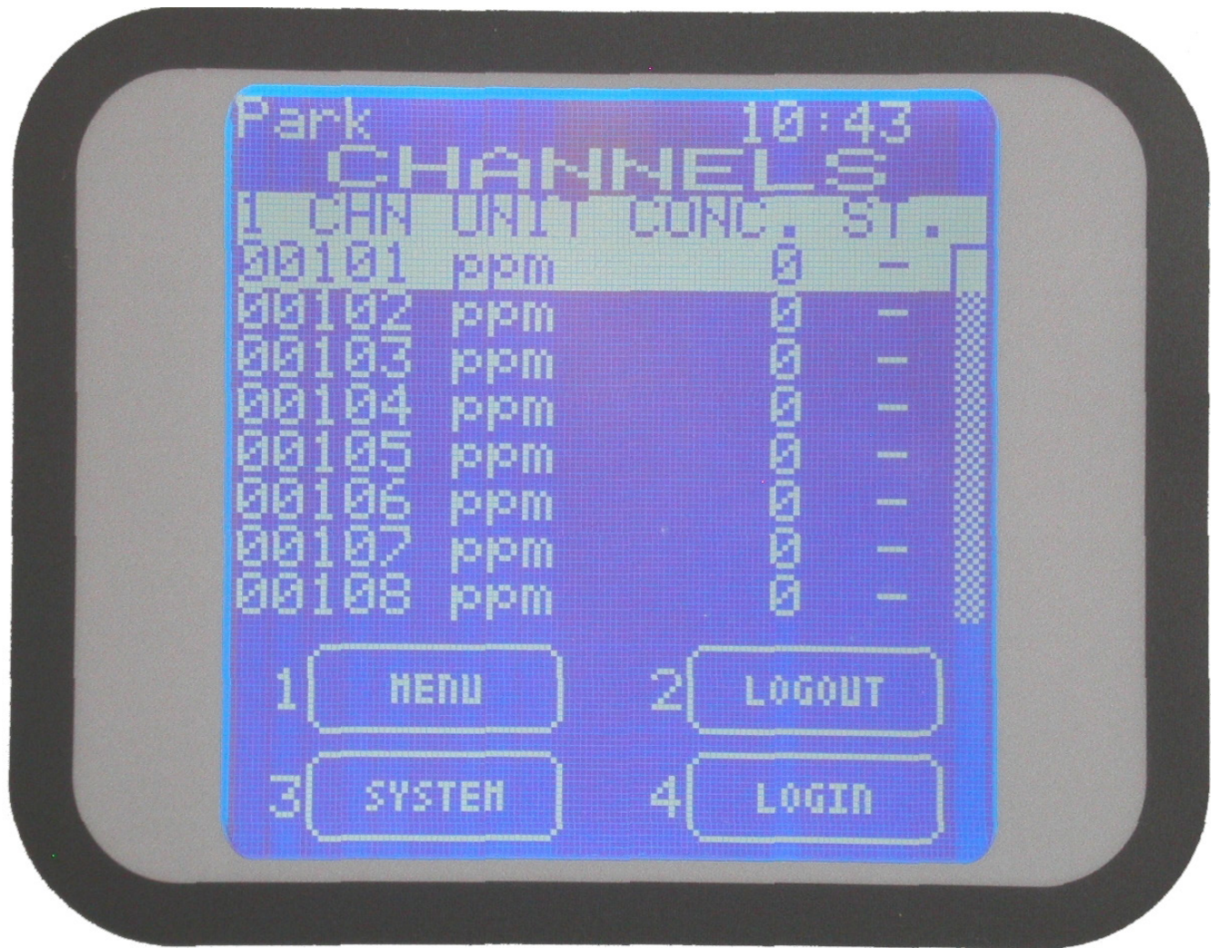
Figure 29 Typical NORMAL state screen
