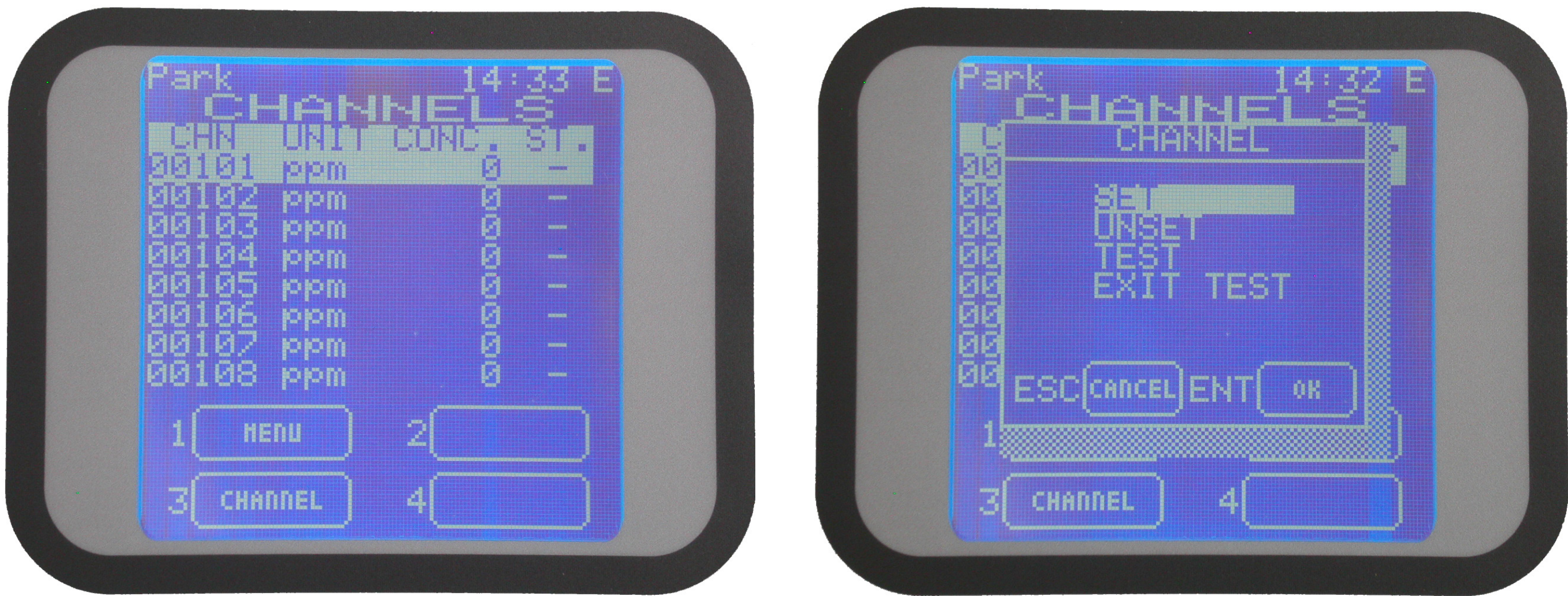
Figure 44 Detectors screen and options available pressing 3-Channel
