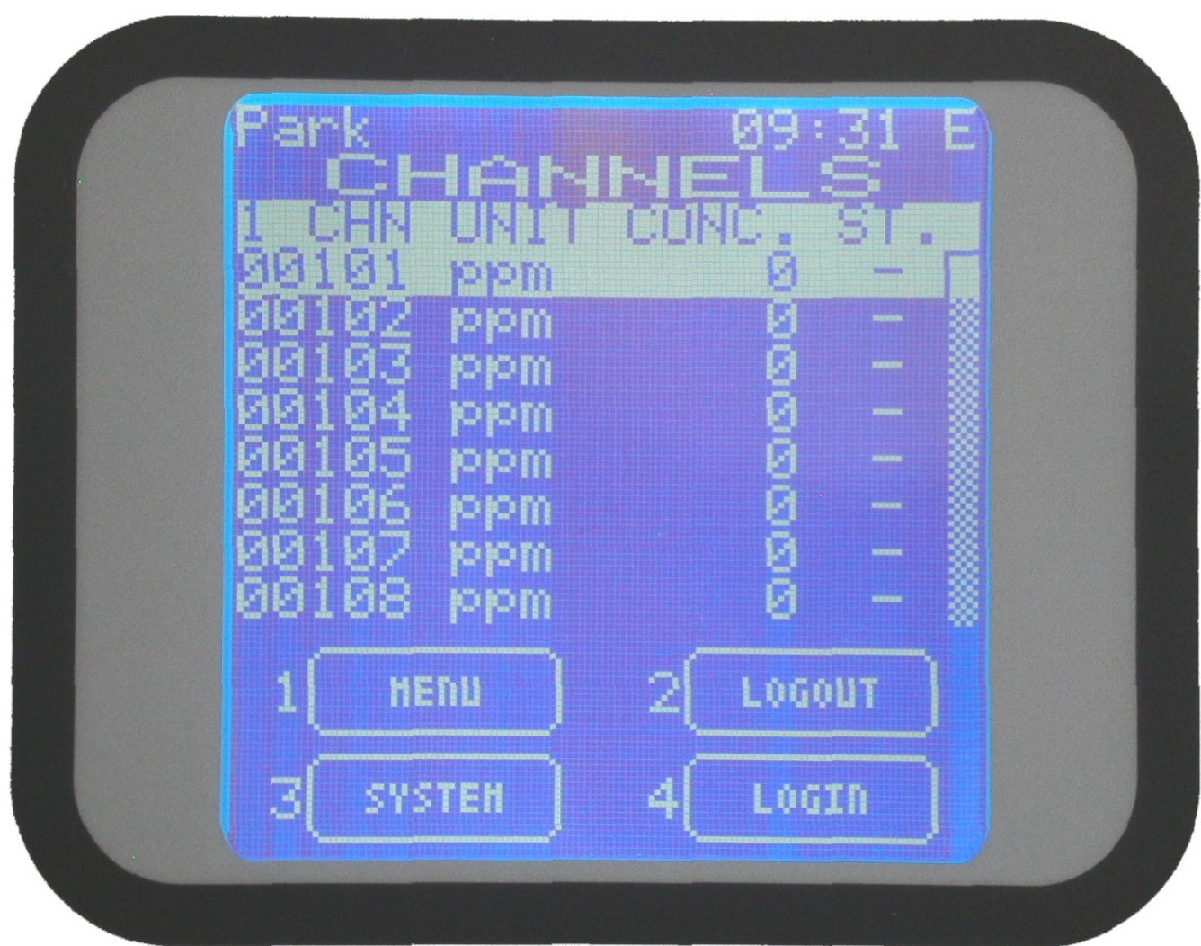
Figure 23 Typical NORMAL state screen.
