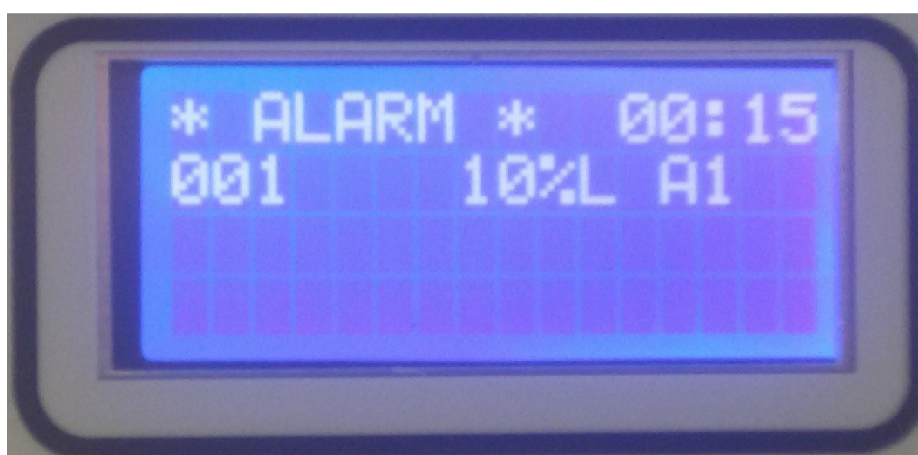
Figure 25 Typical ALARM state screen.
