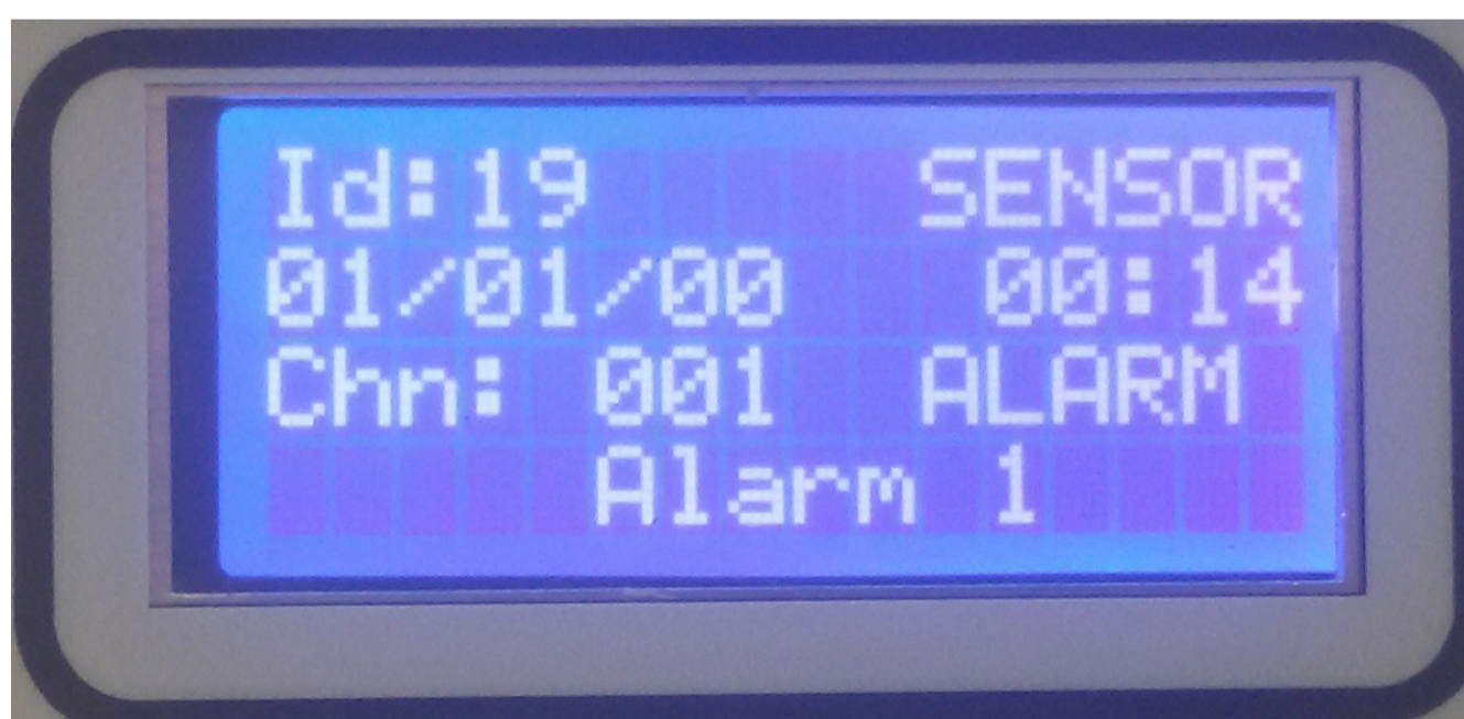
Figure 26 ALARM details screen
