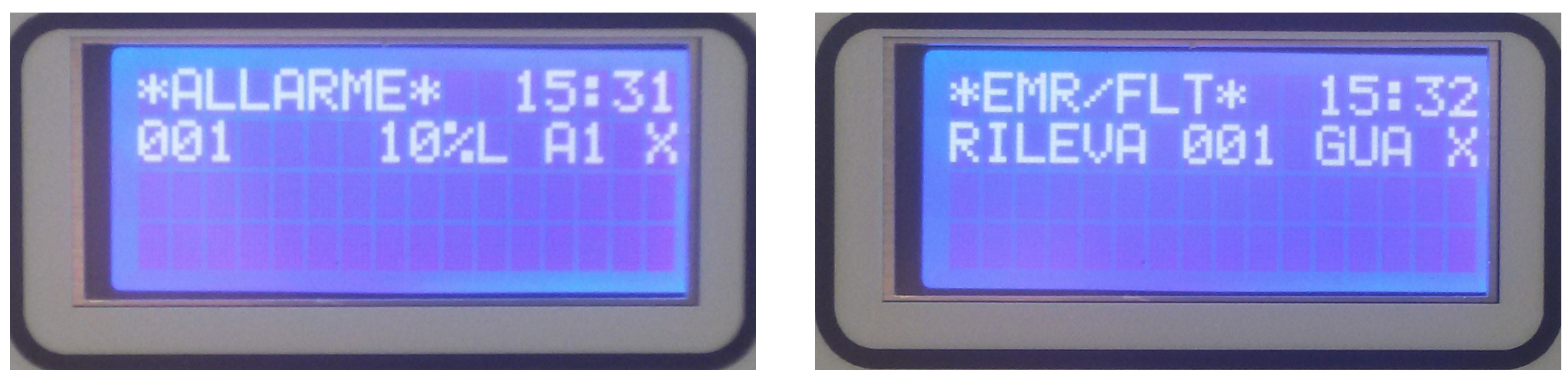
Figure 29 Active Events screen with Alarm and Fault
