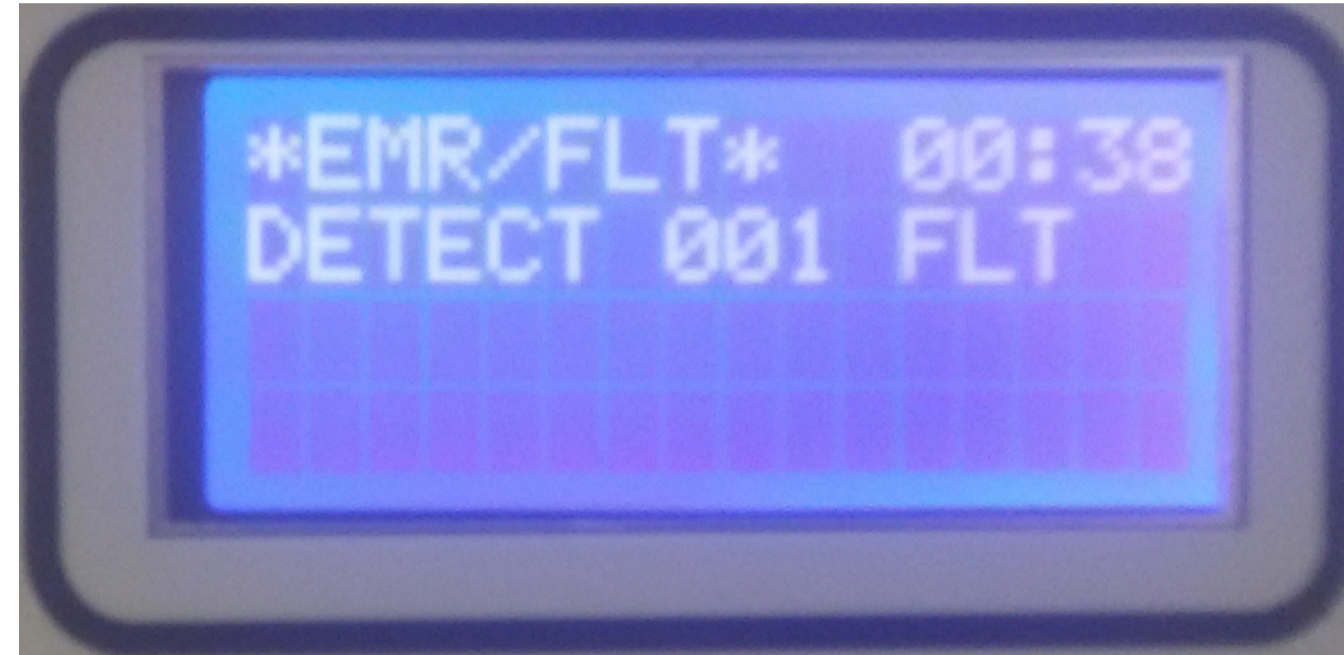
Figure 27 Typical FAULT state screen.
