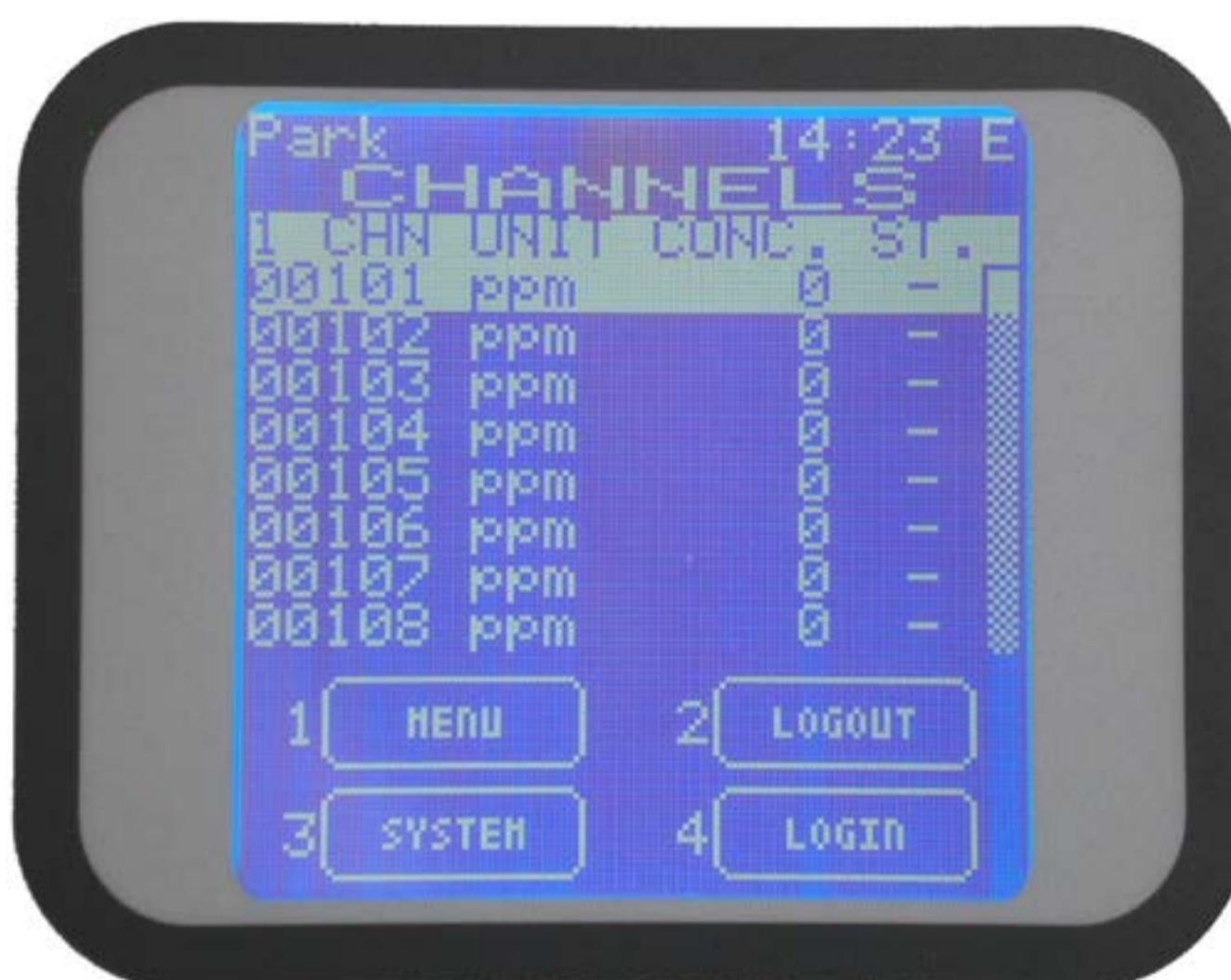
Figure 34 NORMAL state screen with the "E" in the right and upper corner
